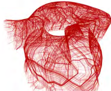
loads distribution on outer surface
