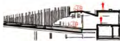
Barrier Elimination Using moats with gentle slop to eliminate the need of physical barriers, allowing a closer encounter between the giant pandas and the visitors.
