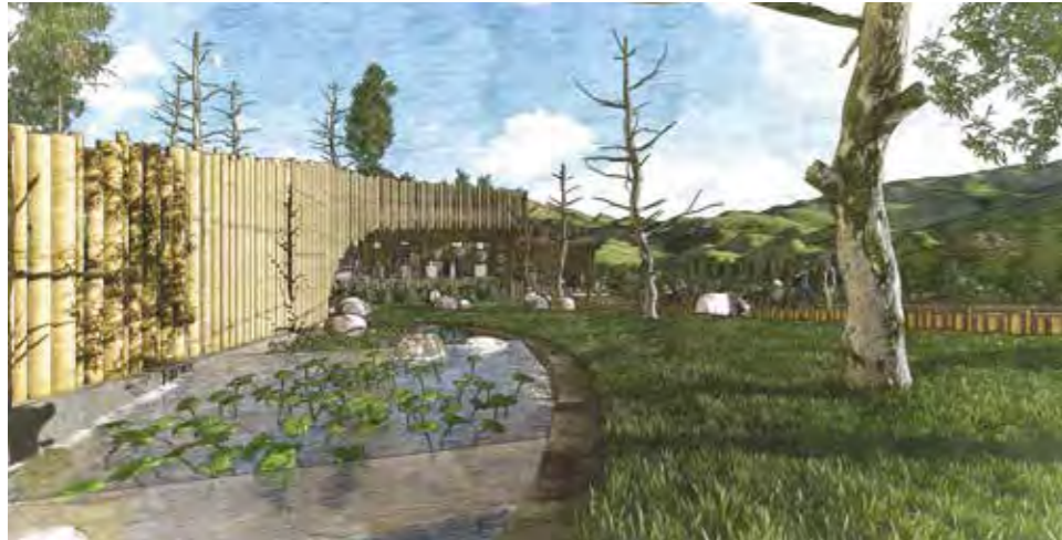
Barrier Elimination Using moats with gentle slop to eliminate the need of physical barriers, allowing a closer encounter between the giant pandas and the visitors.
