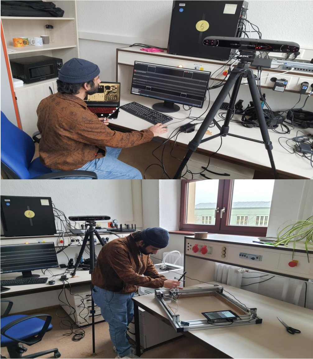
Figure 4.7: Evaluation setup from left to right: ART SMARTTRACK, Performer and Teaching Tracking System.
