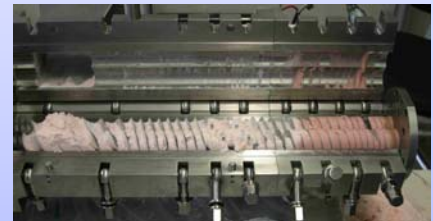
View into the opened extruder showing material in different heat, mix and dispersing zones
