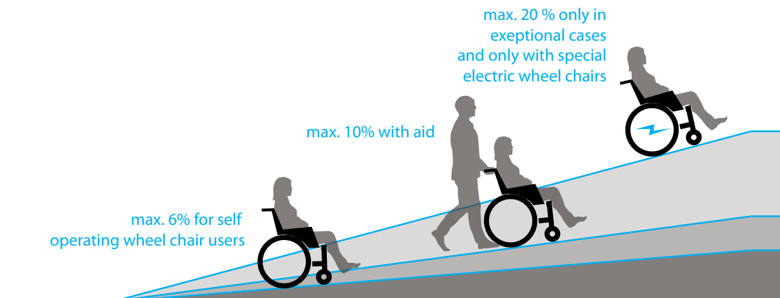
Fig. 69_ Different ramp slopes
