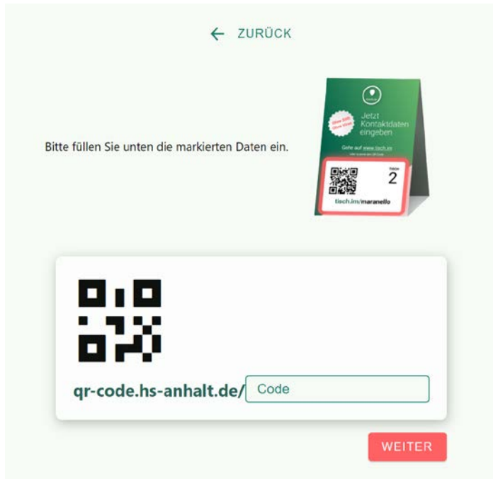
Figure 6: Manual input of the code that is located below the QR code. The location and room designation are stored in it. Upper and lower case is not evaluated.
